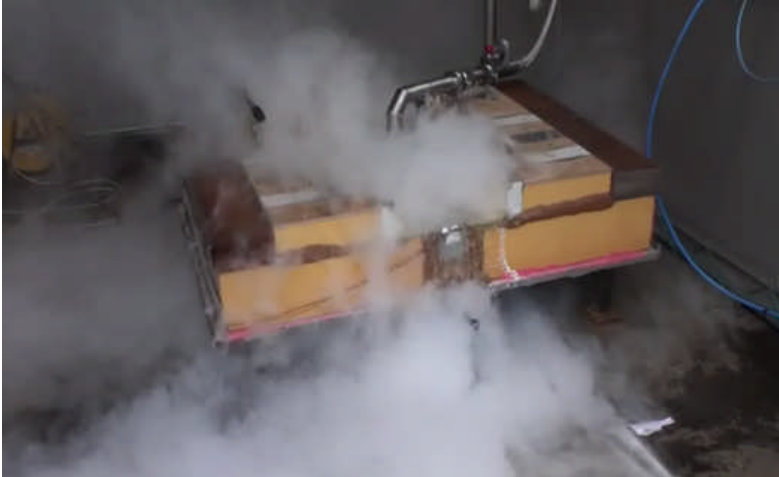
Fig.11 Specimen subjected to hull deformation under cryogenic temperature
